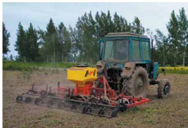
Fig. 1. Combined unit for seedbed preparation and sowing green manure crops
