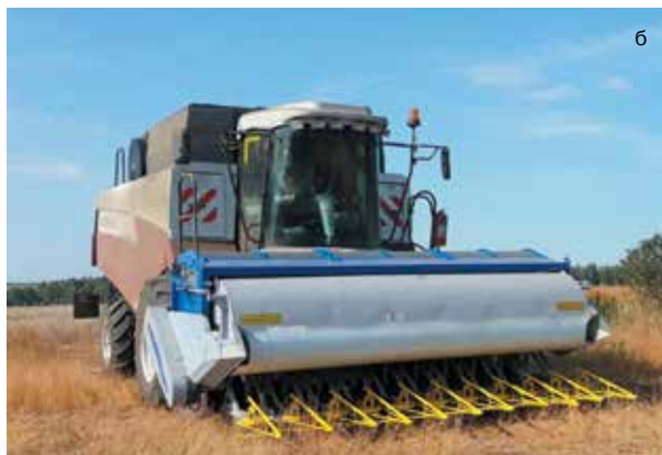
Fig. 1. Multifunctional unit for flax harvesting (a — diagram, b — general view): 1 — grain harvester, 2 — top-lifting device, 3 — stripper, 4 — threshing and separating device
